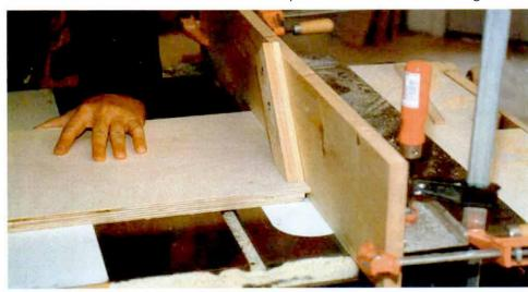
**Cutting the tongues.** A featherboard attached to an auxiliary fence makes the process safer and the tongues more consistent in thickness.
