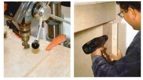
**Hanging doors starts with a drill press.** After testing the layout on scrap, the author drills 32mm holes in the backs of cabinet doors (above left). Pencil marks on the drill-press fence indicate the door-edge alignment. A jig locates screw holes for hinge plates inside the lower cabinets (above right).
